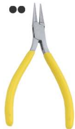
S-803 Round Nose Pliers 120mm Carbon Steel Made Nickle Plated, Box Joint Pvc Handles.
