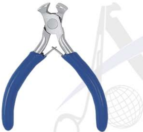
S-950 End Cutter 130mm Double Leaf Spring, Lap Joint Carbon Steel Made, Pvc Handles.
